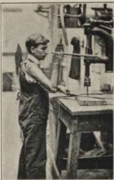
DRILLING WORK FOR SUBMARINE FITTINGS.
