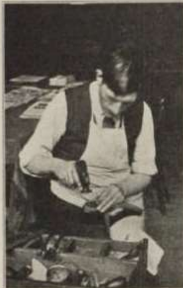
BOOTMAKING BUILDING THE HEEL.
