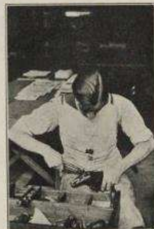
BOOTMAKING. DRAFTING THE UPPER TO THE LAST.
